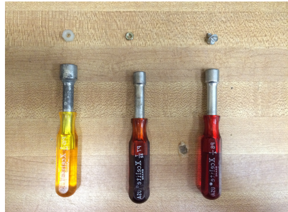
Nut drivers - Yellow for plastic nuts, orange for small metal nuts, red for metal enclosure screws
