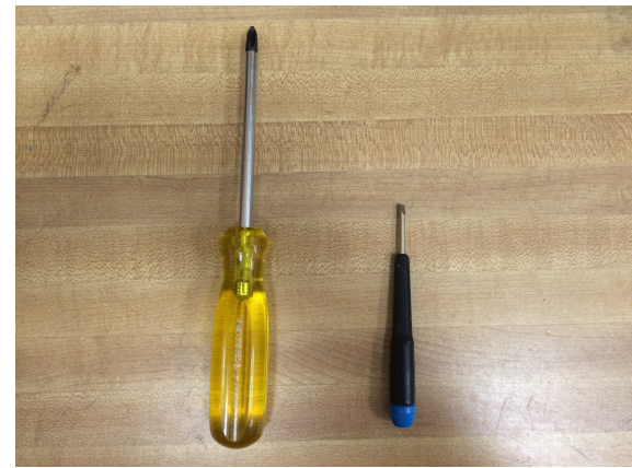
Screwdrivers. The small blue one can be used to adjust potentiometers on LVS and display
